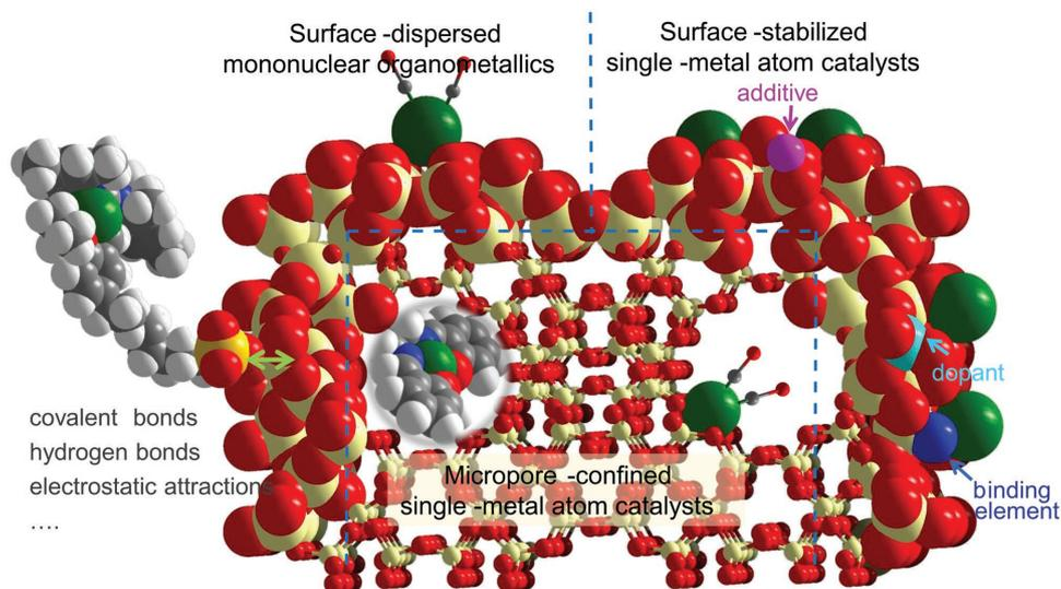
**Figure 1.** Illustration of three different classes of atomically dispersed catalysts. Color codes: green, catalytic metal; yellow, metal of support; cyan, dopant metal; red, O; purple, additive; blue, nitrogen or other binding element; gray, C; white, H.
